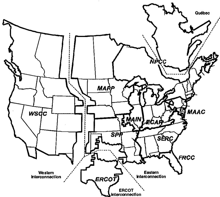
Figure 3. Approximate locations of the 10 regional reliability councils. The Western Systems Coordinating Council (WSCC) and the Electric Reliability Council of Texas (ERCOT) are each interconnections as well as reliability councils. The remaining eight councils are all located within the Eastern Interconnection.
